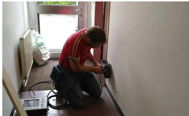
GPR scan of a wall
